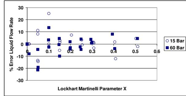
**Fig.5** Self testing - liquid rate accuracy vs Lockhart Martinelli parameter
