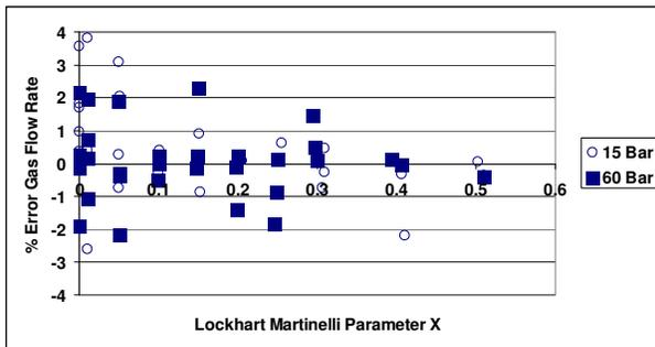
**Fig.4** Self testing - gas rate accuracy vs Lockhart Martinelli parameter
